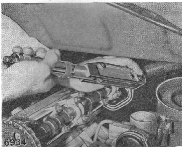
Fig. 38. Churchill spanner RG355 for tightening cylinder head bolts with camshaft in position
