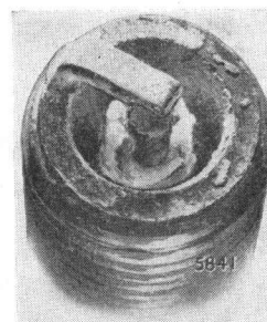
Fig. 12. Burnt or overheated
