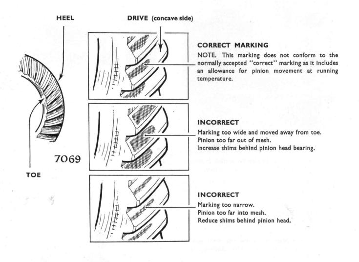
Fig. 47. Crown wheel tooth markings
