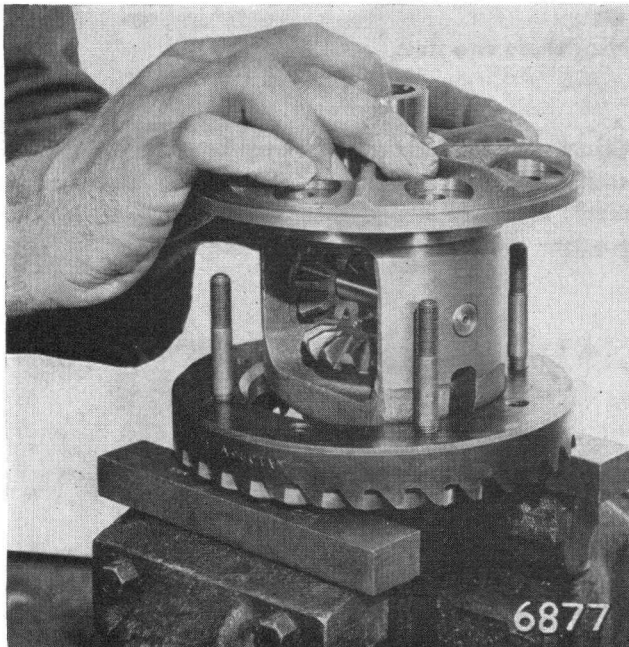
Fig. 40. Fit crown wheel to case
