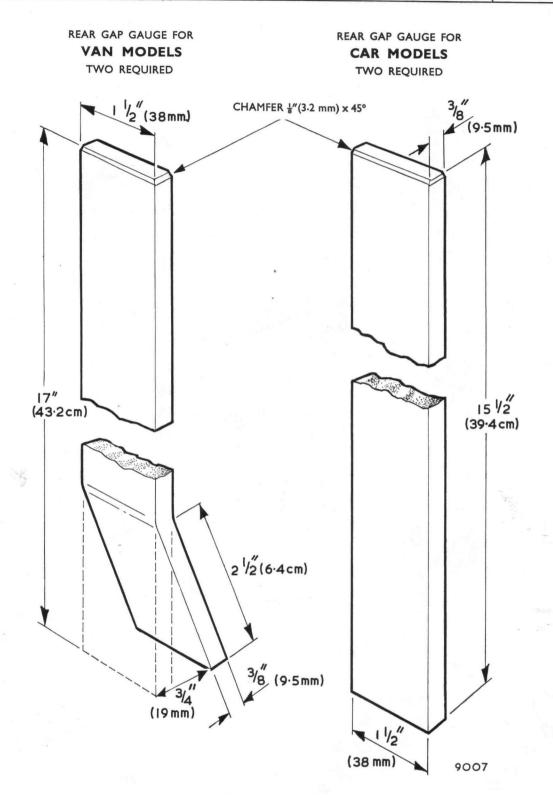
THE ABOVE GAP GAUGES CAN BE MADE IN SERVICE WORKSHOPS FROM MILD STEEL BAR. IT IS IMPORTANT THAT THE GAUGES ARE CHAMFERED AT THE TOP AND REMAIN SQUARED AT THE BOTTOM AS SHOWN.
