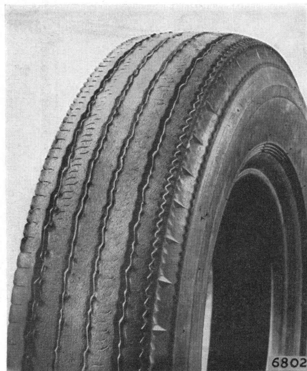
Fig. 2. Fin and feather wear due to extreme wheel misalignment.
