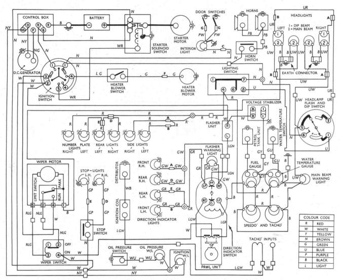
CABLES 'UR' AND 'UW' TO TERMINALS 3 AND 5 RESPECTIVELY ON HEADLAMP FLASH-AND-DIP SWITCH ARE REVERSE CONNECTED FOR LEFT-HAND-DRIVE CARS.
