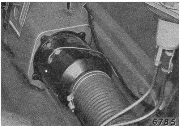
Fig. 2. Blower unit and air hose
