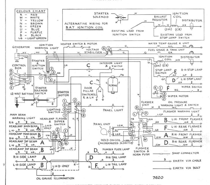
COMBINED BINNACLE-MOUNTED HEADLAMP FLASHER & DIPPER SWITCH IS REPLACED BY A FLOOR-MOUNTED DIPPER SWITCH FOR NORTH AMERICA EXPORT. IN THIS INSTANCE, THE UW AND UR CABLES FROM THE HEADLAMPS WHICH ARE NORMALLY CONNECTED TO THE HEADLAMP FLASHER AND DIPPING SWITCH, ARE JOINED BY IN-LINE CONNECTORS AND THE N LEADS WHICH CONNECT AT TERMINAL SIX OF THIS SAME SWITCH, ARE DELETED.
